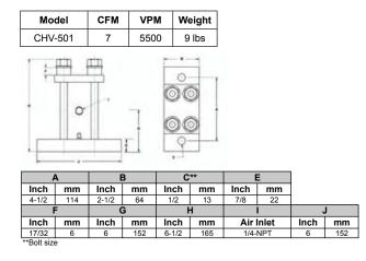
\*Steel mounting channel iron is 30" standard length. Can be cut to custom length.
